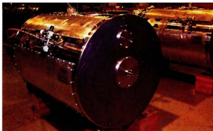
Prototype cryomodules containing superconducting accelerating cavities for CERN's LHC collider.
