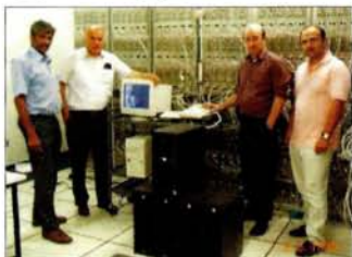
Computing on the Liverpool MAP. Each rack carries 30 PCs and 2 ethernet hubs. Left to right: G Patel, E Gabathuler, A Moreton and T Bowcock. In the foreground is a prototype 1 TByte server on loan from Dell Computers UK.
